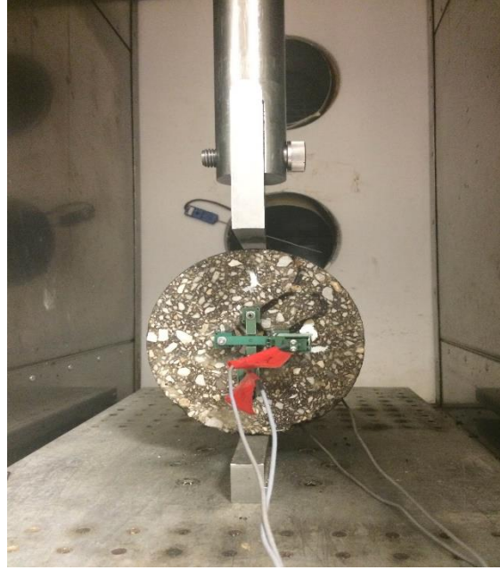
Figure 10. IDT |E^*| Setup
