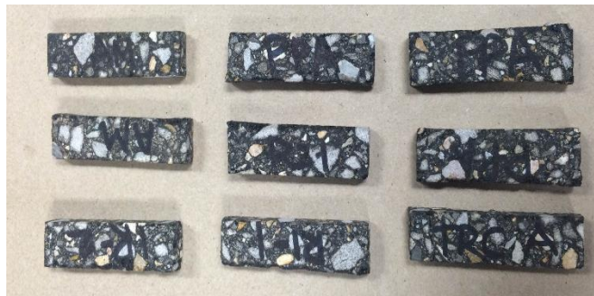
Figure 8. Torsion Bar |G^*| Geometry
