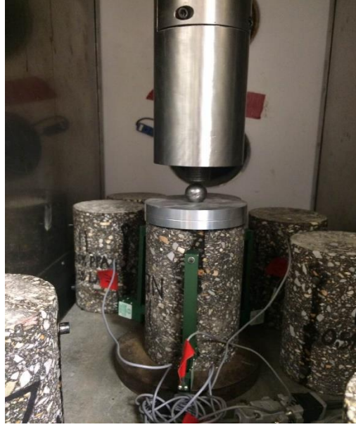
Figure 9. Uniaxial |E^*| Test
