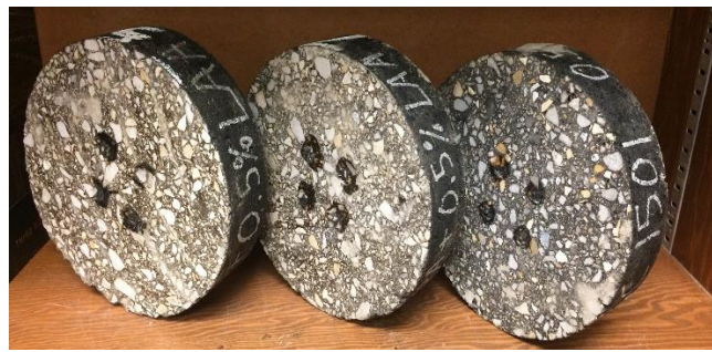
Figure 7. Indirect Tensile (IDT |E^*| ) Geometry
